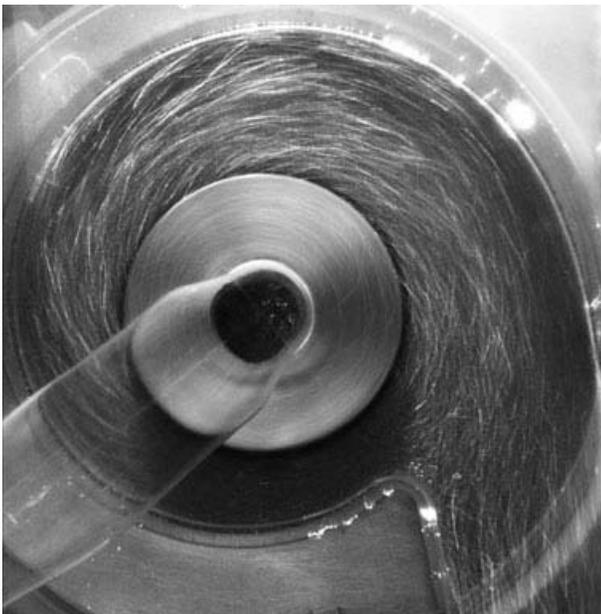
**FIG. 7.** Flows in volute above the impeller shroud: (a) computational fluid dynamics (CFD) prediction; (b) experimental flow visualization.
