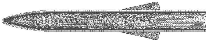
**Figure 6. Symmetry plane of mesh generated around finned-missile**
