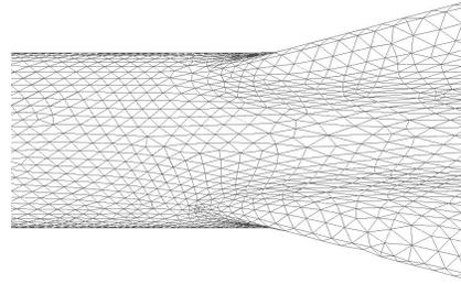
**Figure 8. Detail of mesh outer surface near fin root**
