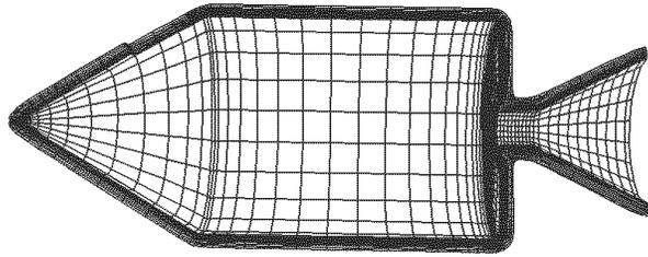
**Figure 3. Symmetry plane of mesh generated around notional Apollo spacecraft**
